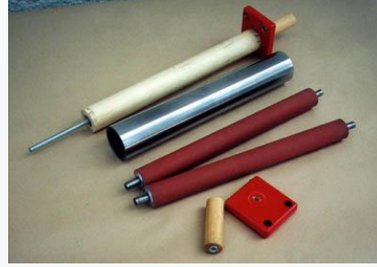
(Three Part Roller for waterless Lithography invented by Professor Nik Semenoff - 1991)
