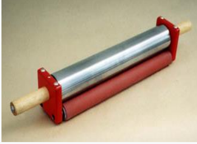
(Three Part Roller for waterless Lithography invented by Professor Nik Semenoff - 1991)
